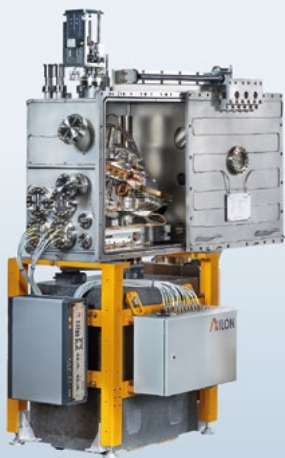
Double-Crystal Monochromator for the APS-Upgrade Project (Argonne National Laboratory)
